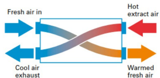
Fig 3: Ventilation process (Source: Northern Fans)
