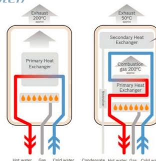
Image: Bosch – Conventional system (left) versus Condensing system (right)
