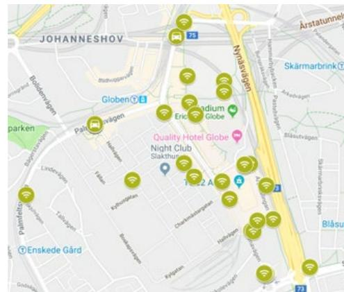
By tracking movements from sensor to sensor, a pattern of movement can be established as well as the volume of moving devices. This can be used to predict people flow within the area.
