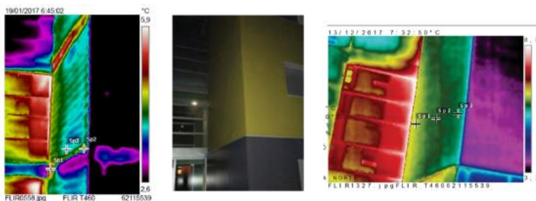
Figure 74 Thermal image of north facade before (left) and after (right) facade thermal upgrade works
